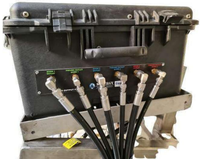
DIVING PANEL WITH D1/D2/D3 INLET (HP/LP) AND OUTLET FITTINGS (TO DIVER) FROM THE BACKSIDE OF THE PANEL
